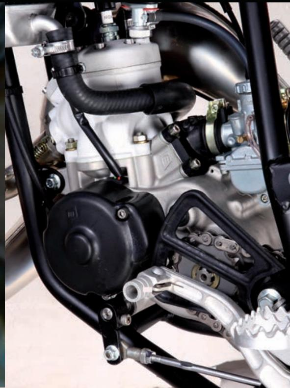
tuned engine – Lawson uses it to boost low-end performance. The ready access to torque means the MT80 can feature just a four-speed gearbox, resulting in a significant weight reduction and increased ease-of-use.
